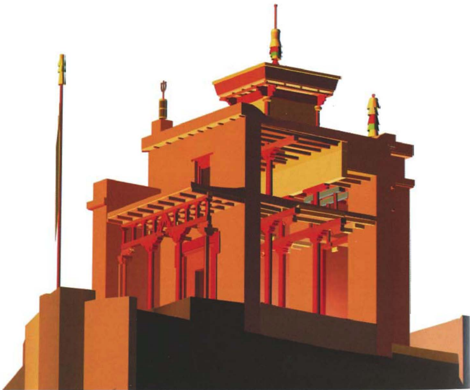
37 Cross section of the Wanla temple (drawing Gerald Kozicz)
